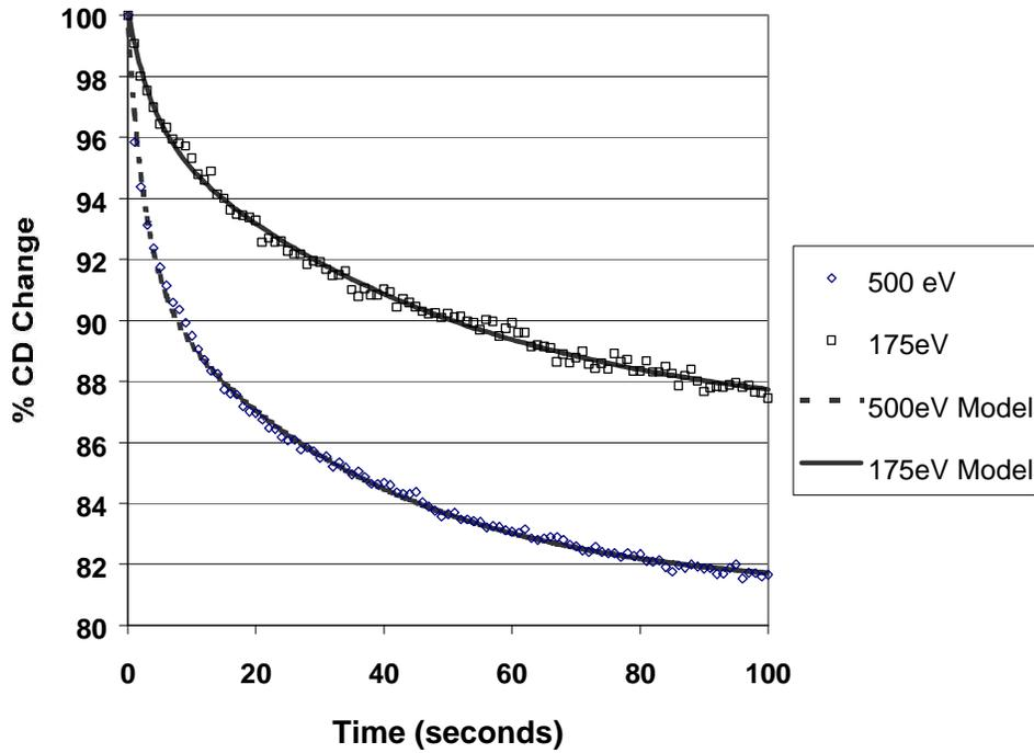
Figure 1: 193 nm resist line width slimming trend
